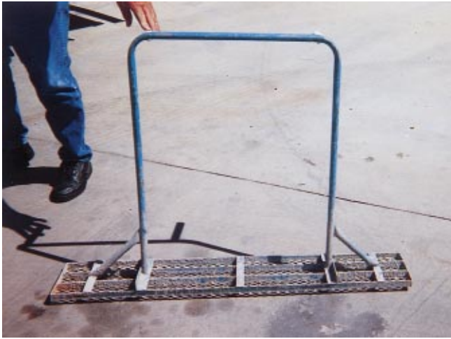
Fig. 8. (Color) Concrete tump like the one used during the tilt-up panel concrete placement
